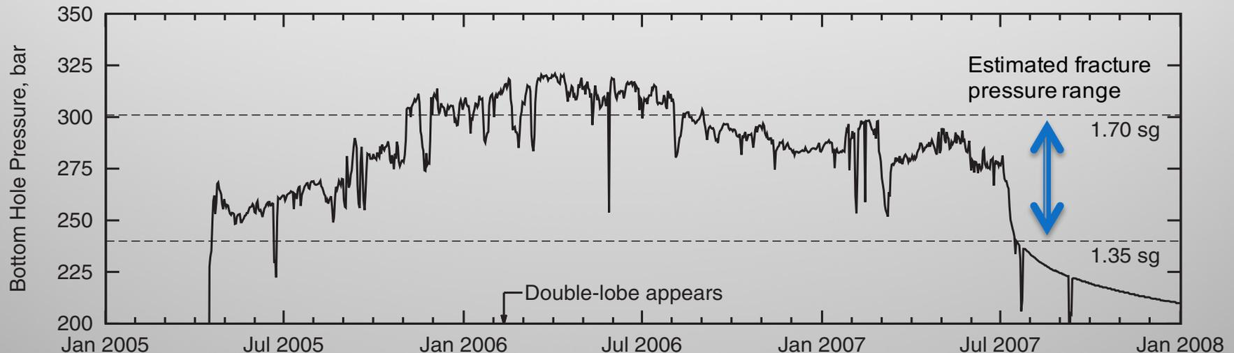
**In Salah Case Study:** Bottom hole pressure and estimated fracture pressure range at KB-502.
