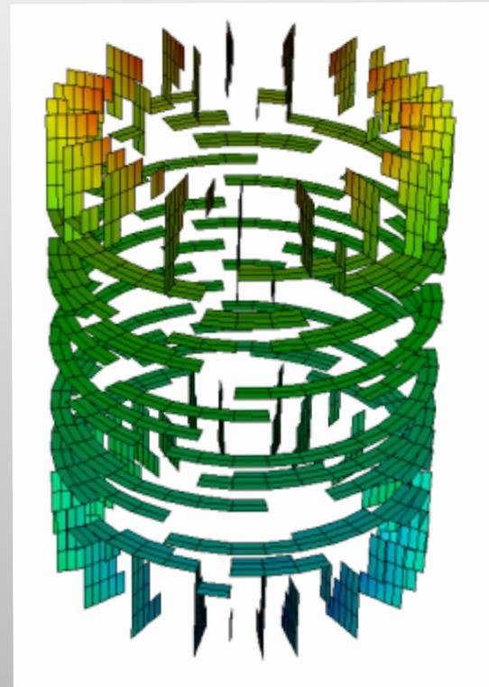
Adding confining pressure slows fracture propagation
