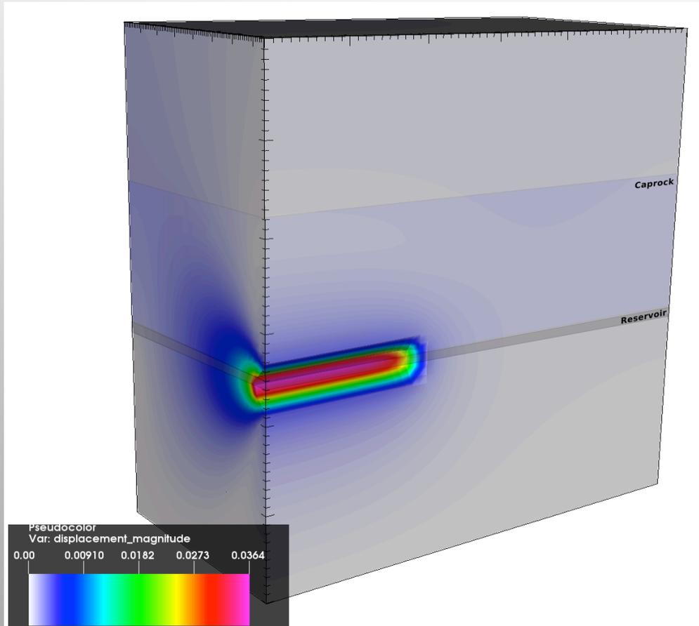
“Static” fracture model used to calibrate rock properties against surface deformation data. Next step will use a propagating fracture to look at the time-evolution of the system.
