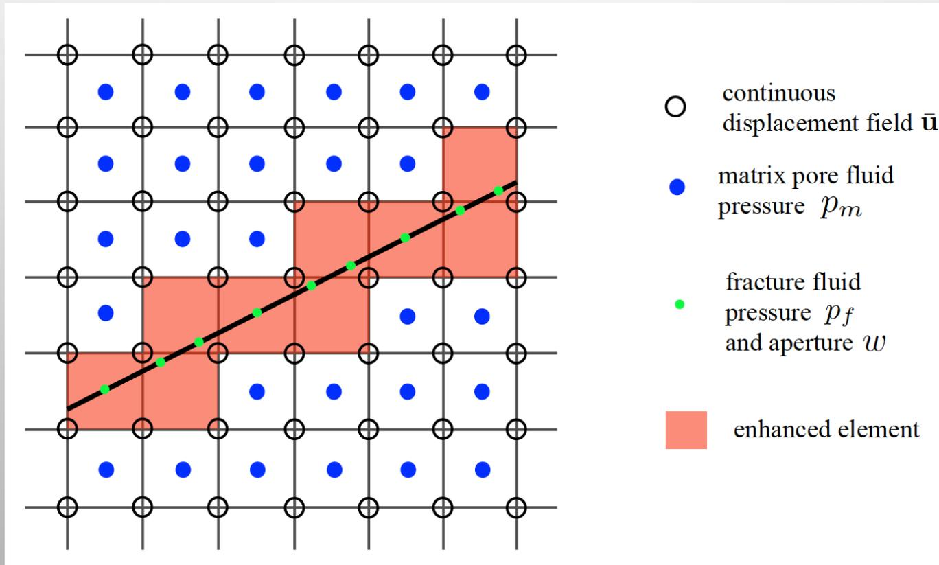
We solve for fracture pressure, fracture aperture, matrix pressure, and matrix displacement in a tightly-coupled fashion.
